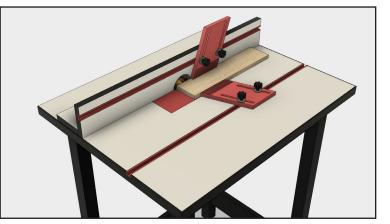
Run each segment through the router table face down. For the best results, use feather boards to keep your work pressed tightly against the table and fence. Feed slowly, and use a push stick to keep your hands at a safe distance from the bit.
