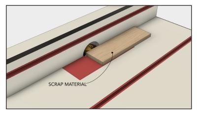
Before routing the segments, run a piece of scrap material through the router. Test the joint's fit.
