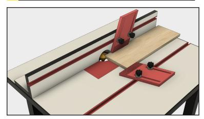
For the cleanest cuts and crisp edges, use a feather board to hold the stock to the router table's surface, and another to press the work into the fence. Feed segments face down for 12-sided objects at a slow and steady rate. A push stick will provide maximum control and will keep your hands at a safe distance from the router bit. **Tip:** Don't cut short segments to length before routing. Instead, route an oversized piece and cut several short segments from it.
