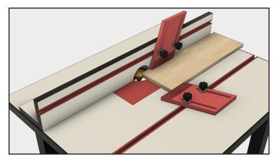
For the cleanest cuts and crisp edges, use a feather board to hold the stock to the router table's surface, and another to press the work into the fence. Feed segments face up for 6-sided objects at a slow and steady rate. A push stick will provide maximum control and will keep your hands at a safe distance from the router bit. **Tip:** Don't cut short segments to length before routing. Instead, route an oversized piece and cut several short segments from it.
