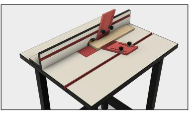
Now you can run your segments face up through the router table. Use feather boards to keep the stock pressed flat against the table and fence. Feed the parts slowly and use a push stick to keep your hands at a safe distance from the bit.
