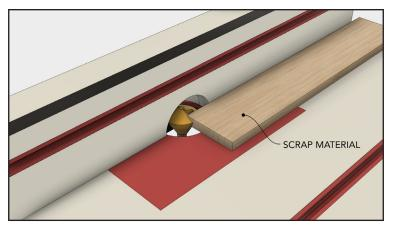
When your bit height and fence are properly adjusted, run a test cut on one edge of a piece of scrap the same thickness as your stock. Be careful to run the piece face up or face down according to the table below. Test the joint's fit.
